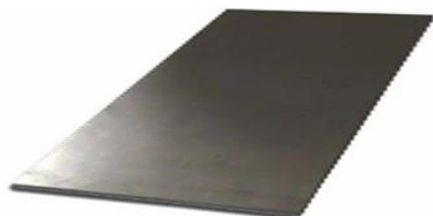
Plate 1: 5.5 x 4 Mild Steel Couple Sample
