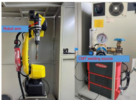
Figure 1. The CMT-WAAM system, including a 6-axis Fanuc robot arm, robot control cabinet, and a CMT power source (TPS400i)
