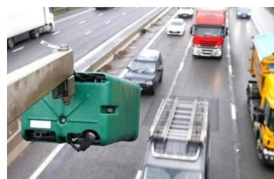
Figure 1. An example of an Automatic Number Plate Recognition (ANPR) system that captures vehicle license plates using Optical Character Recognition (OCR) technology for identification and monitoring purposes.
