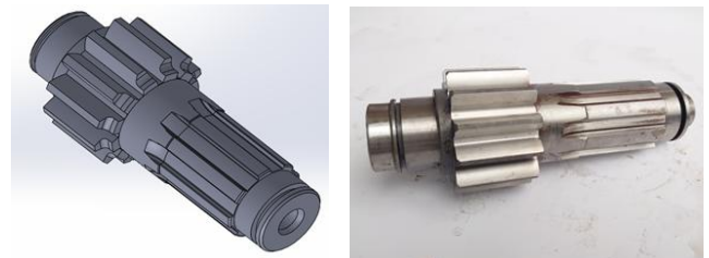
Fig. 3. Shaft and central gear after fabrication
