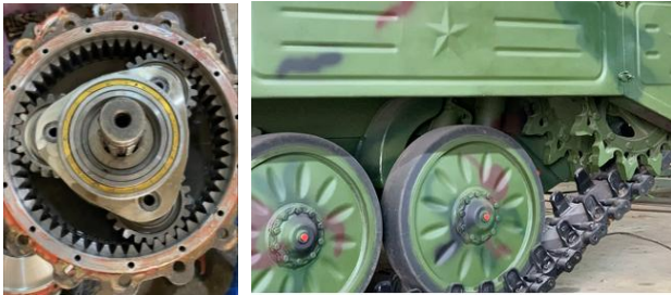
Fig. 5. Gear reducer after assembly and on the XCB tracked vehicle
