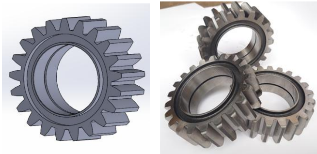
Fig. 4. Planetary gears after fabrication
