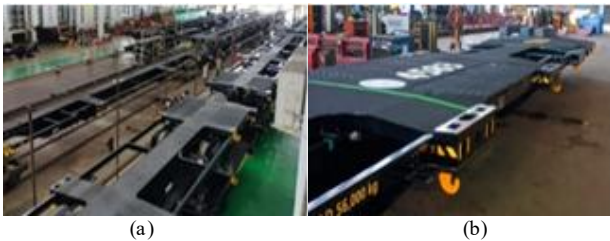
Fig. 1. Container Flat Top Wagon 50 Feet Intermediate Goods (a) dan Finished Goods (b)
