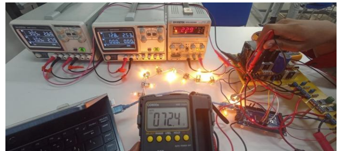
Figure 3.4 Testing Sepic converter with load
