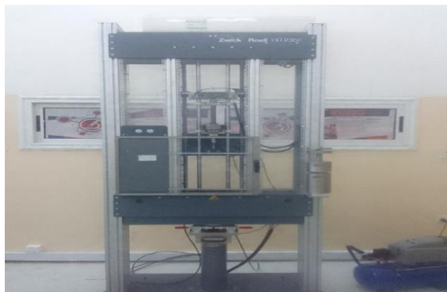
Fig. 3. Zwick / Rolle Hit 230-F Drop Weight Test
