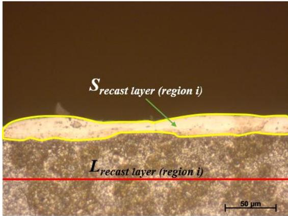
Fig. 2. The method determines  $S_{recast\ layer\ (region\ i)}$  and  $L_{recast\ layer\ (region\ i)}$  by micrograph of the optical microscope in  $i^{th}$  region.
