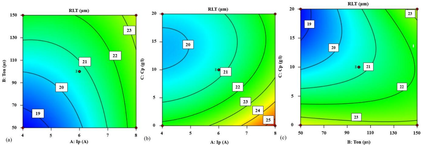
Fig. 4. The incorporated influences of process parameters on RLT: (a)  $I_p$  and  $T_{on}$ , (b)  $I_p$  and  $C_p$  and (c)  $T_{on}$  and  $C_p$ .
