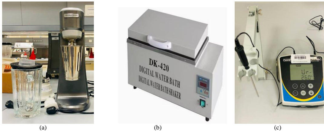
Fig. 1. Drilling Fluid Instrumentation: (a) Electric Mud Stirrer, (b) Water Bath, (c) Electric Thermometer and pH meter
