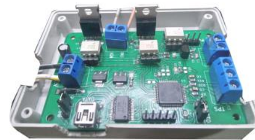
Fig. 2. (a) Mockup Electric Control Unit (ECU) (b) Actual Electric Control Unit.
