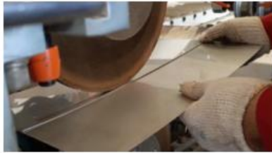
Picture 1. Seam Welding
