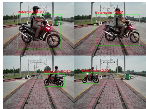
Fig. 9. Result of Motorcycle detection using Object Tracking
