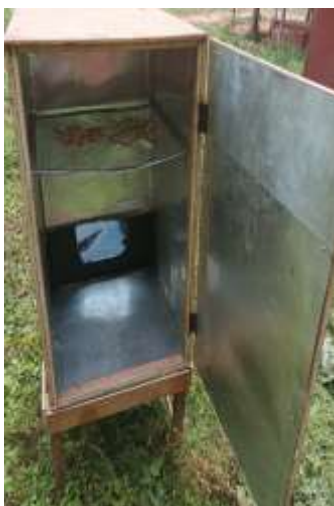
Figure 3a: Drying chamber
