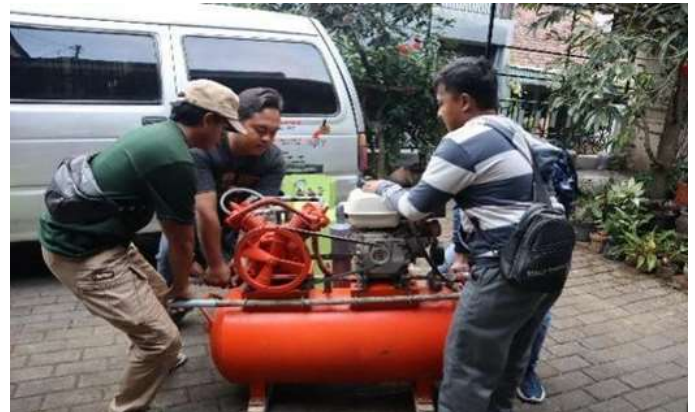
Figure 4. Bovine biogas purification cylinders and compressors
