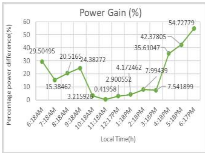
Figure 10: Percentage Power gain as a function of time curve of a 4V PV panel cloudy day March 2nd, 2023.
