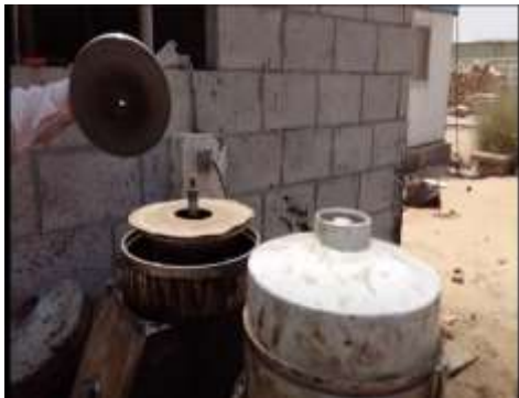
Fig. 16. Bitumen produced by centrifugal force
