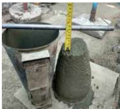
Figure 2. Slump testing of fresh concrete
