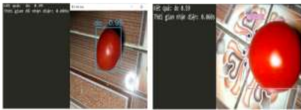
YOLOv3 (P=0.99; Time = 0.089s); Darknet (P=0.59; Time = 0.06s) Fig. 9. Figure 9. Identification of red tomatoes
