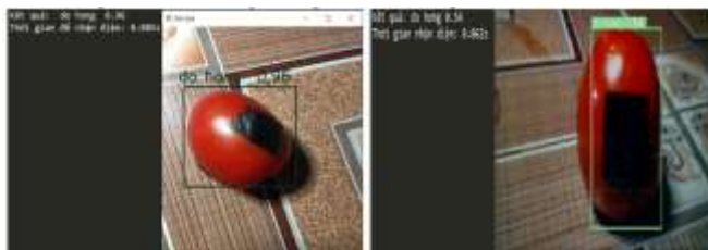
YOLOv3 (P=0.96; Time = 0.085s); Darknet (P=0.54; Time = 0.062s) Fig. 10. Identification of red-failed tomatoes
