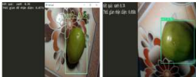
YOLOv3 (P=0.95; Time = 0.077s); Darknet (P=0.74; Time = 0.058s) Fig. 11. Identification of green tomatoes
