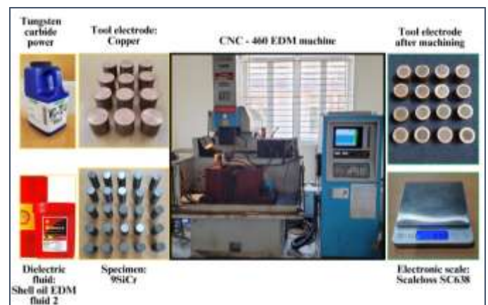
Fig. 3. Machines, materials and tools used in the experiment.
