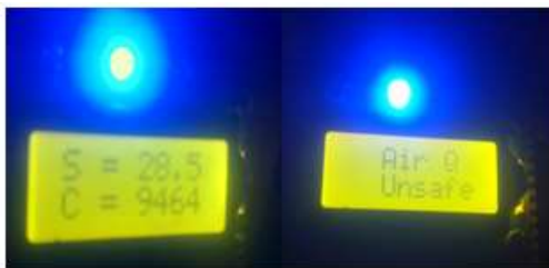
Fig. 7: Second test soot device detected unsafe environment
