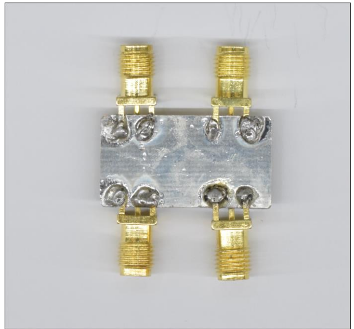
Fig (14): Back side of the module of the cloudy lumped-distributed branch line coupler v2
