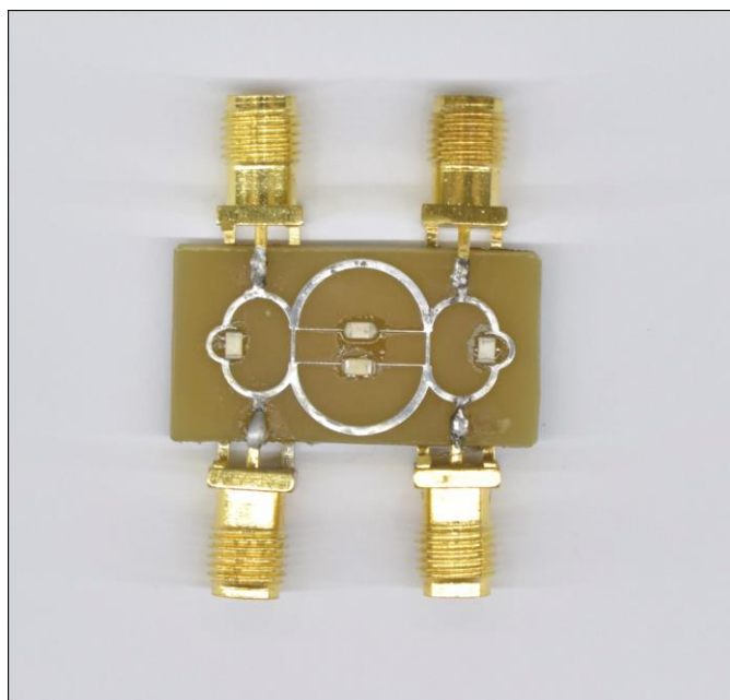
Fig (13): Front side of the module of the cloudy lumped-distributed branch line coupler v2
