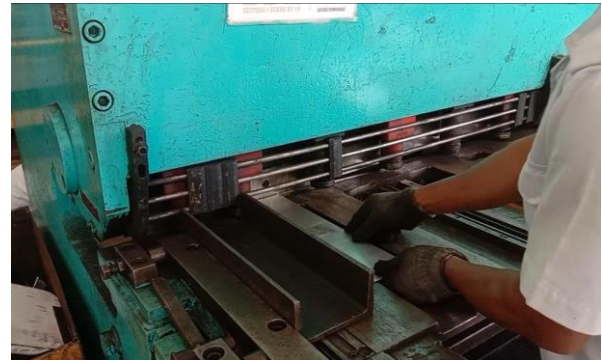
Fig. 1. Process Cutting Materials with Gap Shear Machine
