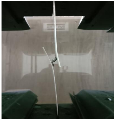
Fig. 3. The Process of Tensile Shear Test
