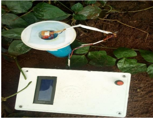
Figure 4: Developed soil infiltration device
