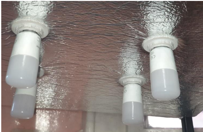
Figure 7. four LEDs placed on the upper plate
