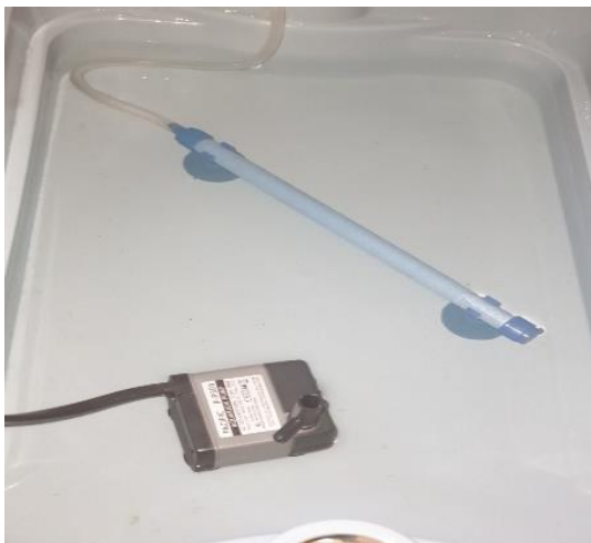
Figure 8. Figure mm Air stone and quarium pump inside the reservoir
