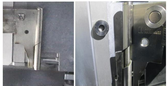
Fig. 5. Automatic Rotary Hinge (ARH) mounted on the output module
