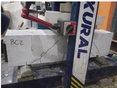
Figure 2. Beam Flexure Test method.
