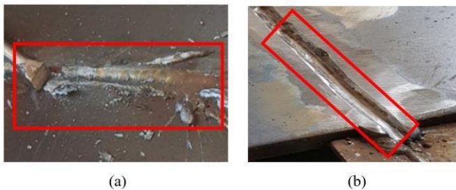
Fig. 6. (a) Specimens After Gouging, (b) Boreback After Gouging
