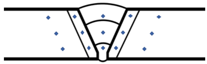
Fig. 5. Hardness Vickers Test Identification Point
