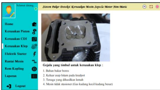
Figure 4.8 Display of the results of the administrator of the valve damage
