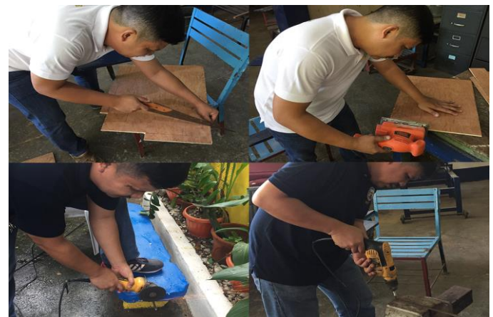
Fig. 3. Cutting, Polishing, Grinding and Drilling of BOJACK’s Materials
