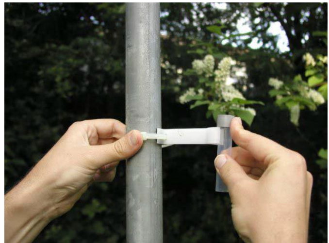
Fig. 3: Deployment of Palme's diffusion tube
