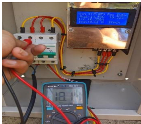
Fig. 18. Measurement of the generator output voltage to the converter
