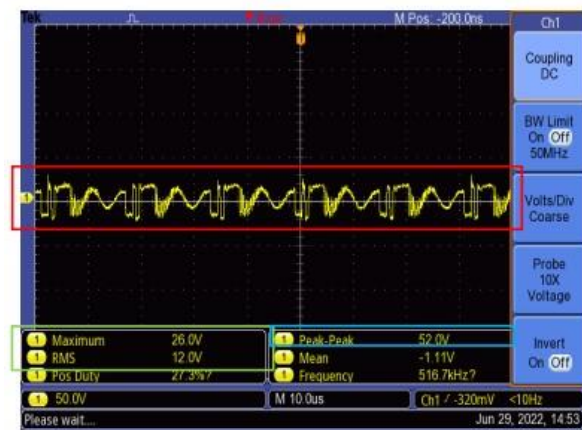
Fig. 8. Converter output waveform measurement.
