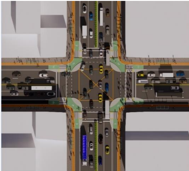
Fig. 1. A Proposed Design of a Bike-Friendly Protected Intersection between A. Soriano Avenue and Juan Luna Avenue Extension, Cebu City.
