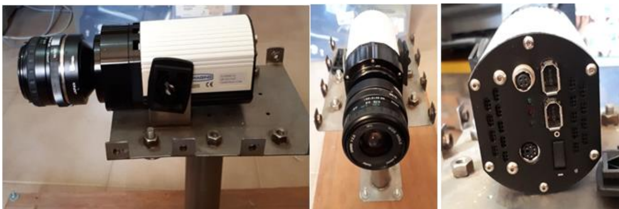
Fig. A1.2 CCD QICam QImaging® with Sony® ICX205 progressive-scan interline CCD monochrome.
