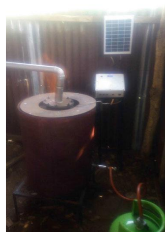
Fig. 2. Gas-fired furnace with attached solar-powered temperature sensor
