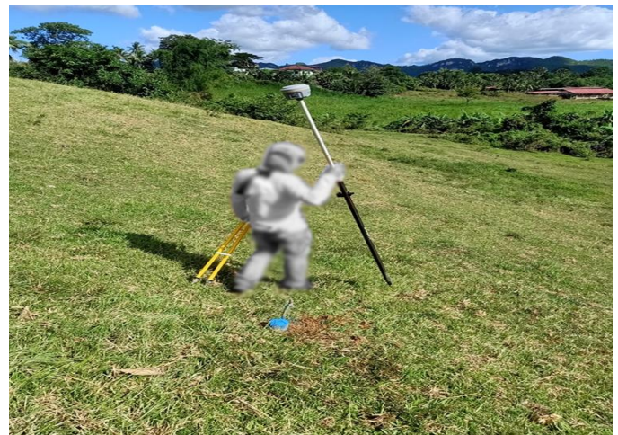
Fig. 25. Setting of points by using RTK rover
