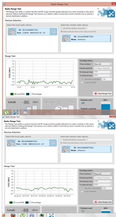
Fig. 10. Radio range test using X-CTU GUI software at 90
