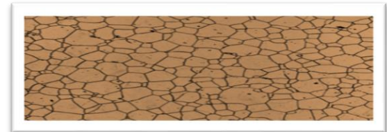
Plate 1c: Grit 120 Coupon for Stainless Steel Coupon (SS 321 VERY ROUGH X500)
