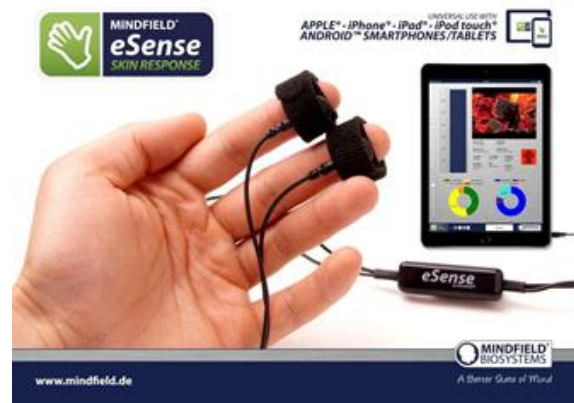
Fig. 6. Mindfield eSense Skin Response EDA sensor
