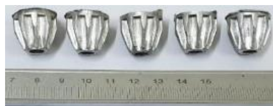
Fig. 13. Experimental forging of bevel gears in closed die
