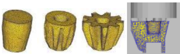
Fig. 6. Metal flowing in cold forging of the straight bevel gear
