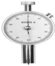
Fig. 3. Shore A instrument
