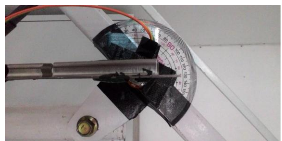
Fig. 4. Test the angle of inclination using a bow
