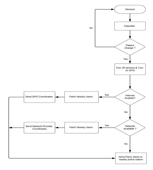
Fig 3.1: Workflow of Embedded Sensor Alert System
