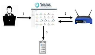
Fig. 2. Flow of Scanner using Nessus
