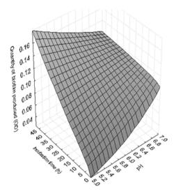
Fig. 2: Effect of pH and incubation time on biofilm formation by *S. aureus* on PVC material
