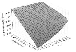
Fig. 1: Effect of pH and incubation time on biofilm formation by *S. aureus* on stainless steel material
