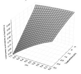
Fig. 3: Effect of pH and treatment time on the probability of biofilm resistance at 60°C on stainless steel
