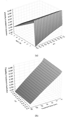
Fig. 4: Effect of NaCl and pH on the probability of biofilm resistance at 60 °C at a fixed treatment time value (7 min) (A) and of pH and treatment time at a fixed value of NaCl (4%) (B) on PVC material.
