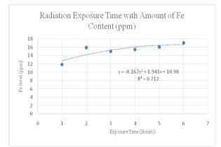
Fig. 2. Relationship between exposure time and total iron content (Fe).
