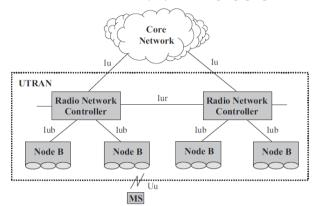
Figure 1: Architecture of UMTS Network [14](Lindemann et al. 2002).
