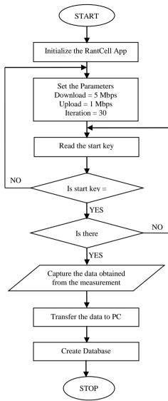
Figure 2: Data Acquisition Flowchart
