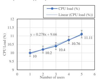
Fig. 6. Linear relationship of the number of users and CPU Load.
