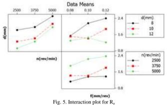
From the graph in Fig. 5 shows: The interaction between drill bit diameter and feed rate has the greatest effect on surface roughness, followed by the interaction between drill bit diameter and spindle speed, the interaction between spindle speed andfeed rate has the least effect on surface roughness.
