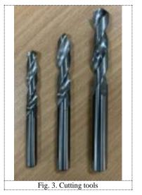
The cutting tool used in the experiment is WIDIN (Korea) hard alloy drill bits with sizes of diameter of 8, 10 and 12 mm (Fig. 3). This type of drill bit is commonly used for aluminum drilling.
