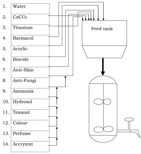
Figure 1: Flow Chart for the Mixing of Paint
