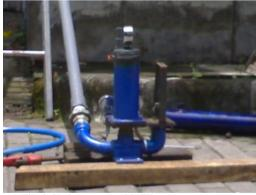
Fig. 2. Hydram pump with IKL pump arrangement
